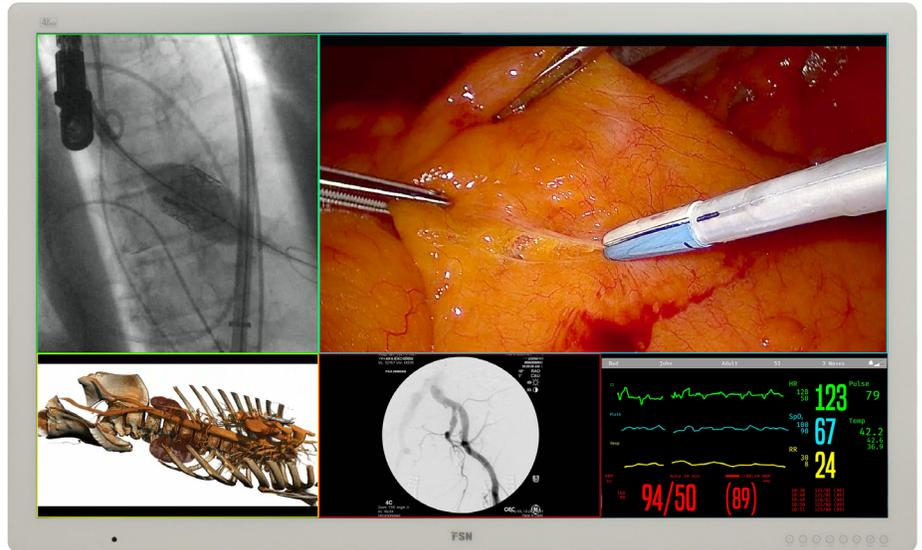
FSN has expanded its range of medical grade monitors to include FM-D5801DV, a large-area display designed to handle a vast array of tasks in the OR from patient monitoring to endoscopic images to X-ray and ultrasound. The FM-D5801DV can show multiple screens at the same time on its large surface area. A flush-front protective glass overlay allows for easy cleaning.
